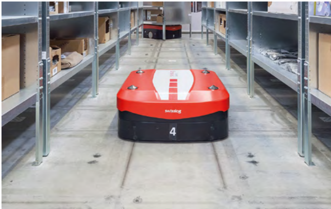
Figure 29: Goods-to-picker concept; Source: Swisslog
